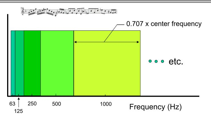
Each octave band filter has a fixed *center frequency* and is twice as wide as the one before it. Each octave band filter may be divided into three one-third octave band filters for more frequency resolution.
