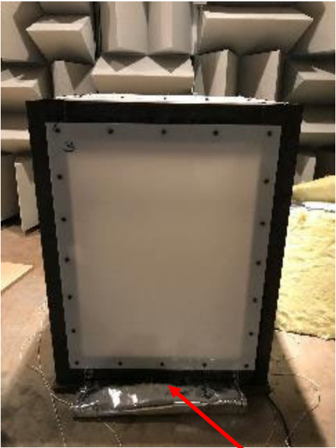
Cavity gap is blocked by lagging material
